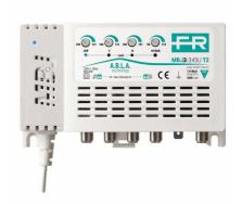
3-input (III+DAB, UHF, UHF) multiband TV indoor amplifier with 20dB gain and up to 115dBµV output level on UHF band, separate amplification with independent level adjustment (20dB) for each input and low noise figure. T2 technology with UHF cut band for LTE 4G @790MHz and 5G @694MHz.
